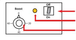
The on/off button gives you hot water for as long as it is kept in the 'on' position.
